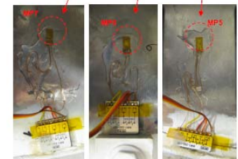
Picture: strain gage measurements on pole claws
