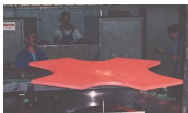
Hot forming with hydraulic press
