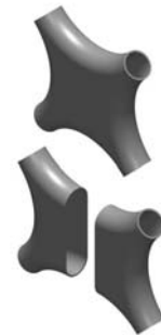
Splitting X-node into two K-nodes
