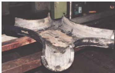
Hot forming with hydraulic press
