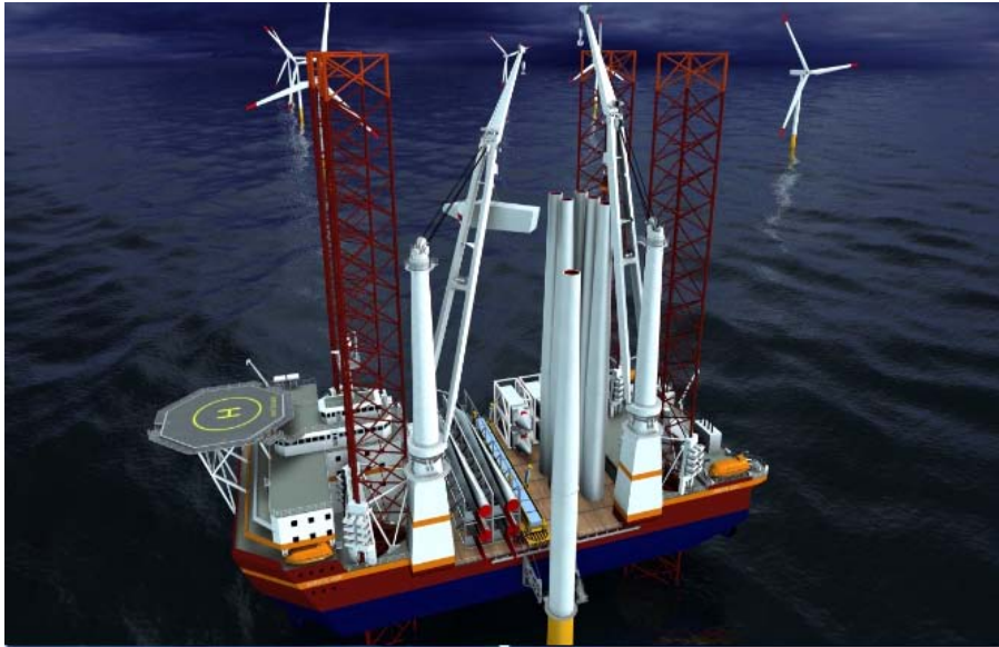
Master Marine – under construction for Sheringham Shoal work
